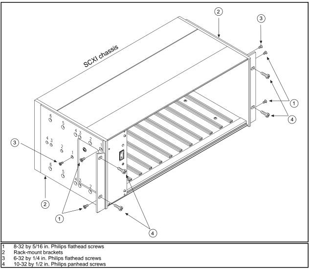
Figure 1. SCXI-1370 Rack-Mount Bracket Installation
